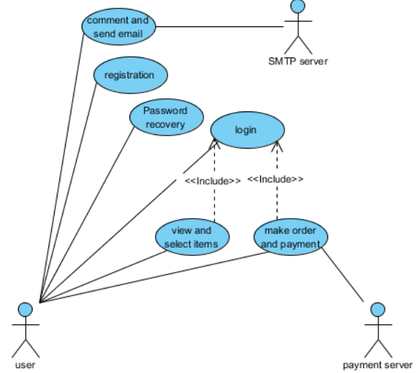
Fig. 7. Use case diagram of the shopping software system
